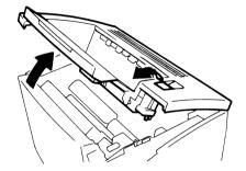
2 Remove the old Imaging Cartridge from the printer.
